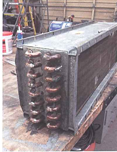
Location: Residential Building 436 Backlog No.: N36-08-436-M-042-1 Deficiency: Severe deterioration of heating distribution system
