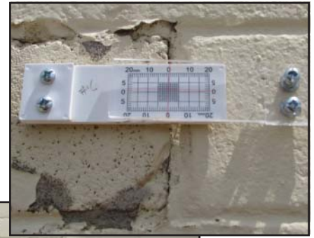
Waconda and Crutchfield locate the monitor (above) that measures cracks in the wall of the Laguna Elementary School gymnasium.
