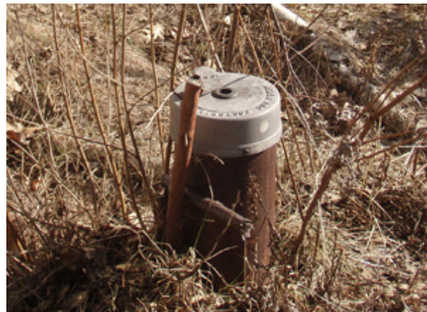
Water Monitoring Well, Keweenaw Bay Indian Community
