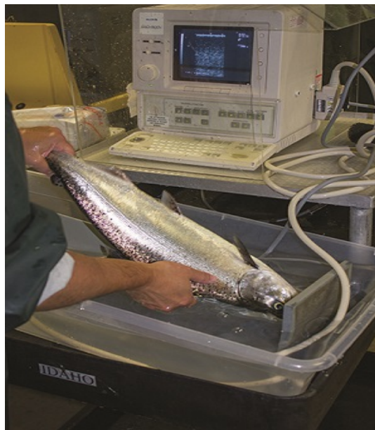
Ultrasound of Nooksack River salmon to determine sex and if ready to spawn
